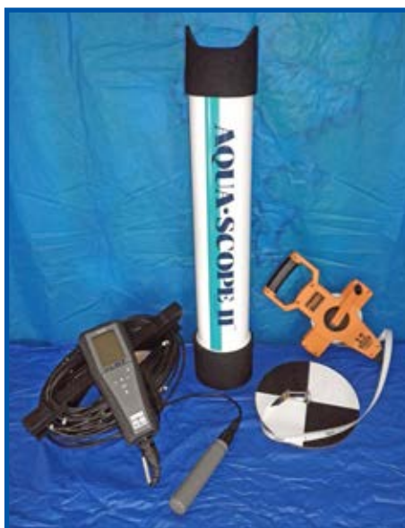
Water quality monitoring 'tools of the trade' (L-R): dissolved oxygen meter with probe, view scope, and Secchi disk with measuring tape.
